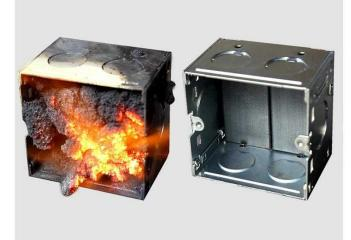
RPBHB is made of high grade special expandable graphite raw material, will expand when exposed to fire and close up the flush box to prevent the flame and hot gas spreading through the wall.
