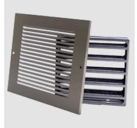
RESSA grille consists of the aluminum alloy frame and graphite based intumescent material core in the middle. When meet fire the pull spring will recover its elastic function because of the easy melting plate of grille will start smelt and break.
