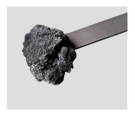
When meet fire or exposed to high temperature, product will expand to seal the gap between glass and curtain wall profile to and prevent the flame and heat spreading.
